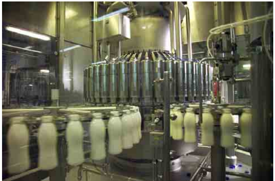
This volumetric filler comes in six diameters with up to 120 valves.
