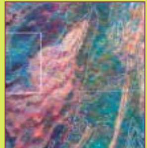
▲ Figure 4. A more sophisticated classification of the Coonawarra gamma-ray spectrometric data, showing most of the major classes of soil in the region. The terra rossa soils are depicted in red tones. Note the generally good correspondence with the Penola Land System (white outline) mapped by the South Australian Department of Primary Industries and Resources.
