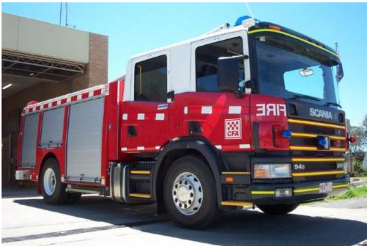
The front looks familiar, the back looks familiar but this is the first time they've been put together. The CFA's new Scania fitted with a body the same as the NSWFB's Isuzu Type 2 pumpers. Photo by Neil Crawley.
