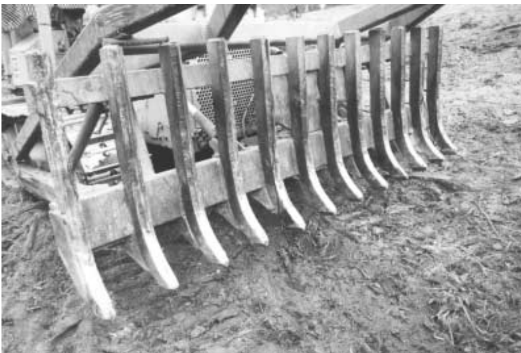
Figure 2 A suitable heavy duty root-rake fitted to a bulldozer. Tyne spacing is 30cm. 1995
