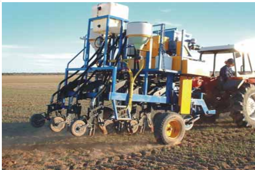
Fluid fertiliser plot seeding equipment used at the Minnipa Agricultural Centre. The plot seeder was designed by Brendan Frischke, SARDI, to apply two separate fluid fertilisers at the same time.
