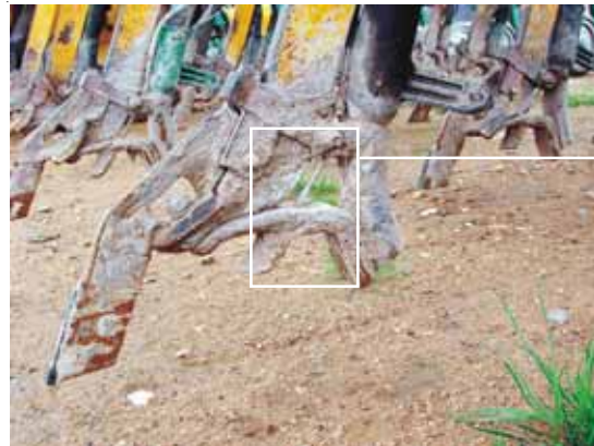
Tyne assembly showing fluid fertiliser injection tube.
