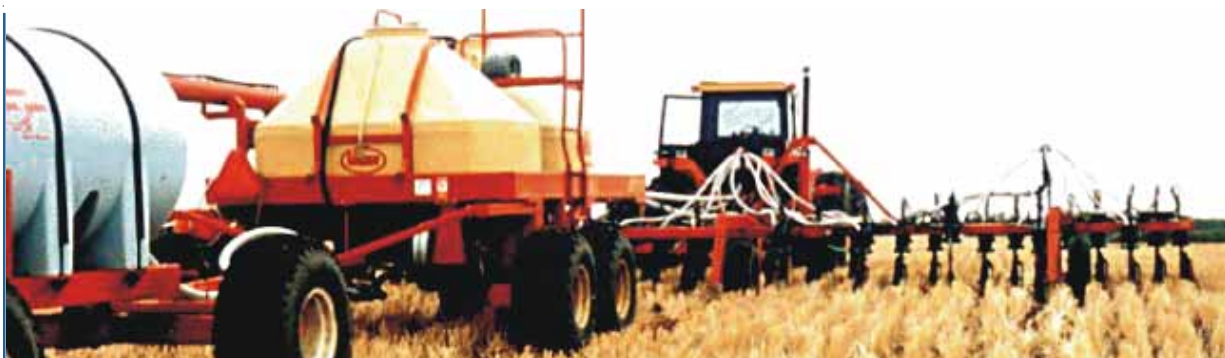
Seeding equipment modified for fluid fertiliser injection
